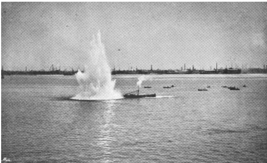
Explosion of a spar torpedo
