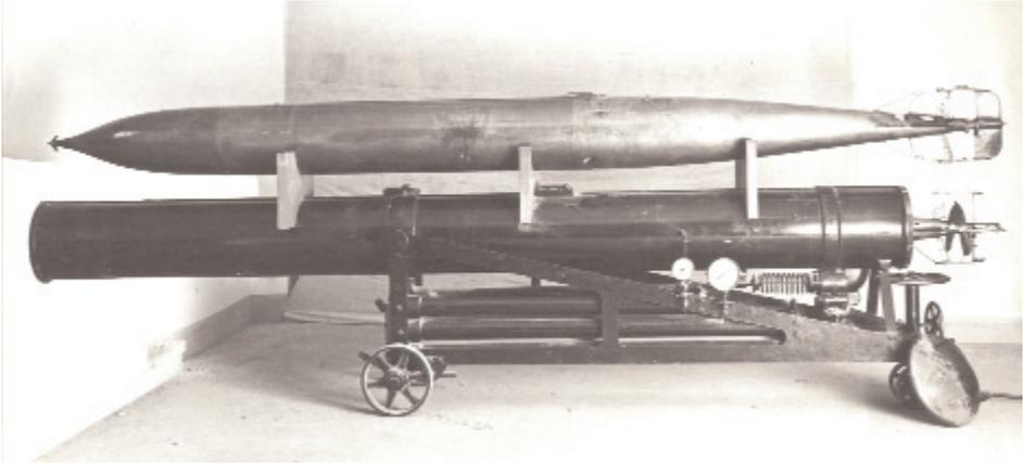
Fig 5: Torpedo C/84A, on top of a launching tube (built by Whitehead, date unknown) with Torpedo C 77.<sup>11</sup>
