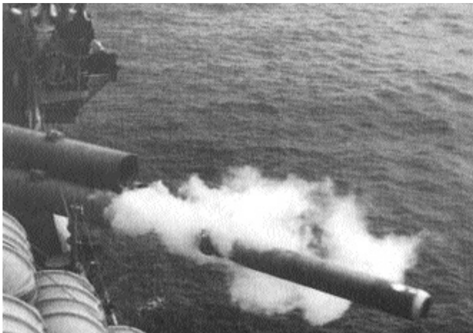
Fig. 55: Launch of a Mk-44 torpedo manufactured by Whitehead Moto Fides (1966 - 1967) (WASS Historical Archive).
