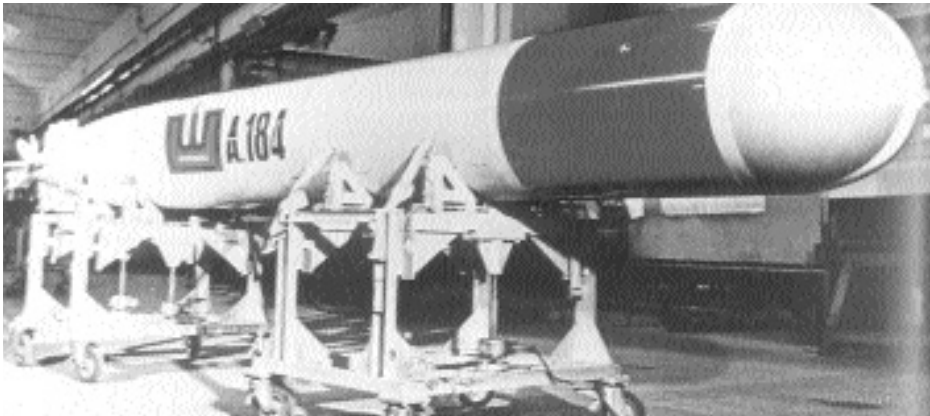
Fig. 60: A.184 dual purpose torpedo (Anti surface ship and antisubmarine). Equipped with electronic wire guidance and acoustic homing (in service since 1978 with several technical improvements) (WASS Historical Archive).
